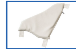
Side filler pads, Laterally velcroable The seat width can be adjusted by attaching it to the inner wall of the chair. The thickness is 30 mm and the inner padding consists of three 10 mm thick panels so that it can be adjusted in 10 mm increments on each side.
