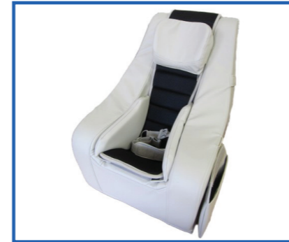
Side filler pads, Laterally velcroable The seat width can be adjusted by attaching it to the inner wall of the chair. The thickness is 30 mm and the inner padding consists of three 10 mm thick panels so that it can be adjusted in 10 mm increments on each side.
